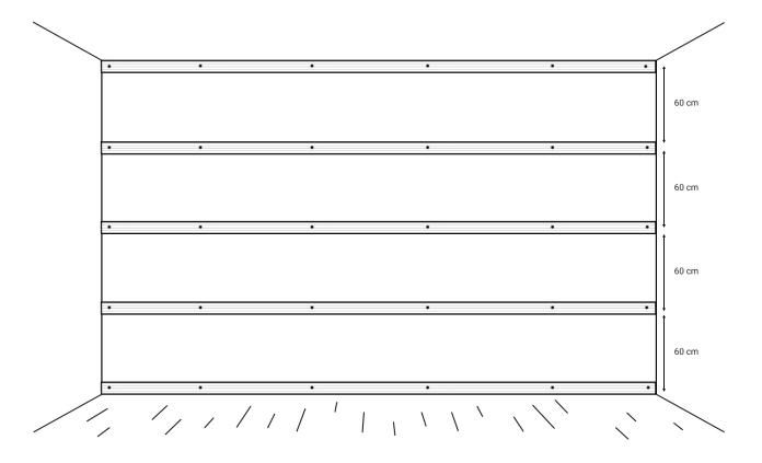
The first thing you need to do is to mount battens on the wall. This enables you to drill the screws through the felt of the akupanels and into the battens. Depending on the wall you will need plugs and and screws that fits accordingly to your wall type. We recommend that you keep a distance of 60 cm. between the battens.
