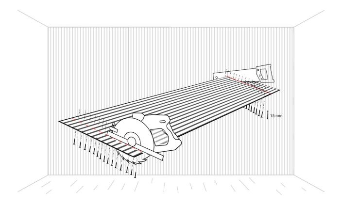
If you need to adjust the height of the Akupanels you can do so by using a saw like for instance a circular saw or a foxtail. Mark the cutting line on the panel with a pencil.
