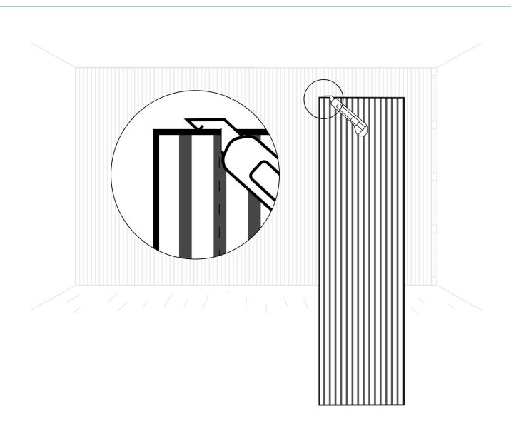
Adjusting the akupanels sideways is done by cutting the panel in the felt using a knife.
